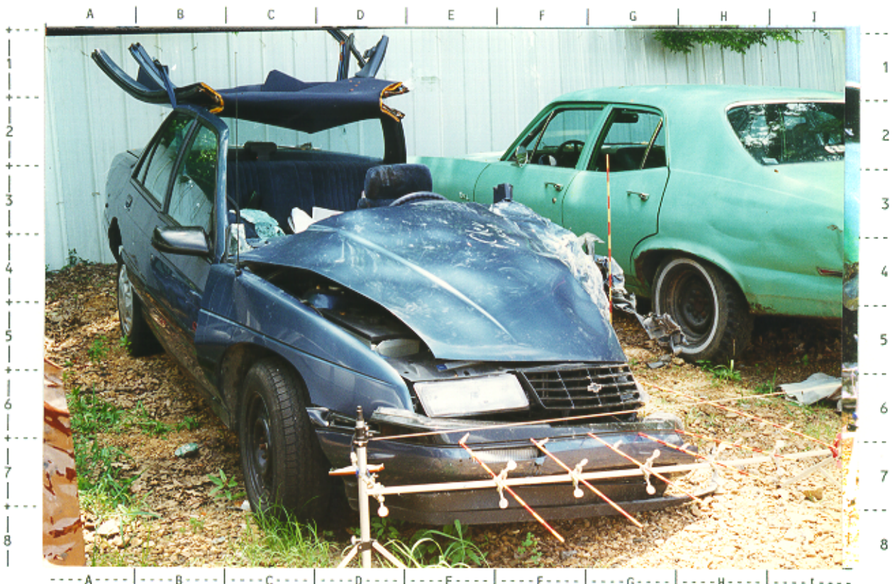
# 46 -- Front right view of frontal and extensive front left damage to 1991 Corsica; NOTE: peeled-back roof and undamaged RF A-pillar
